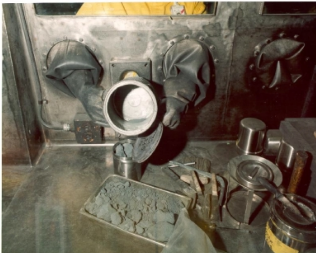
Figure 1. Sampling of a Typical MSE Salt Contents of Container is Emptied into Pan for Examination in the Glove Box
