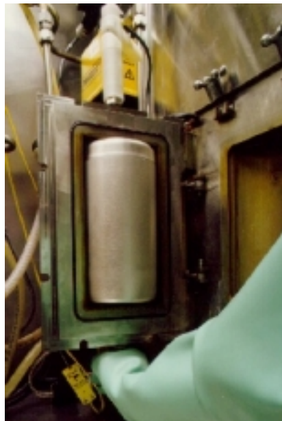
Figure 2. Inner container decontamination fixture and decontaminated storage container as viewed from the "cold" segment of the glovebox.
