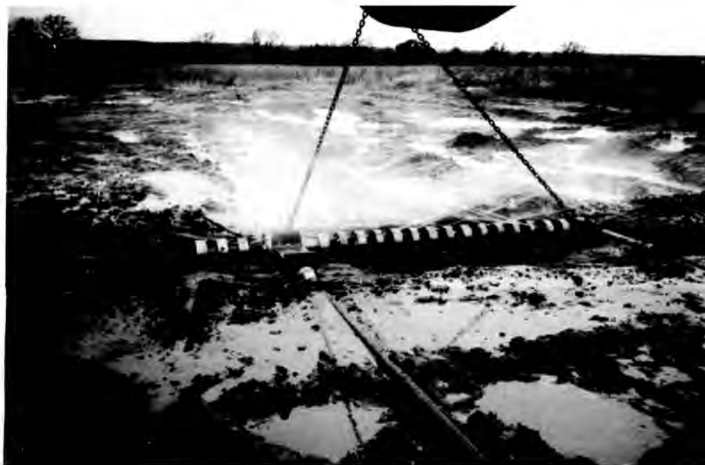
Fig. 2. Jet grouting tool (bar) for horizontal use.
