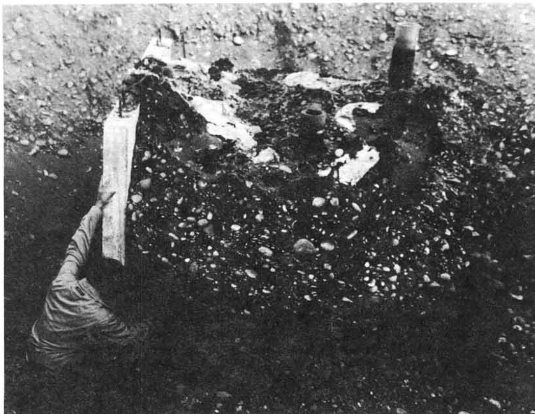
Fig. 5. Vitrified block resulting from pilot-scale test of underground tank vitrification.
