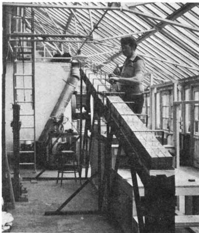
Fig. 22. Large soil beam used for final selection of diatomaceous earth as conductive layer material.
