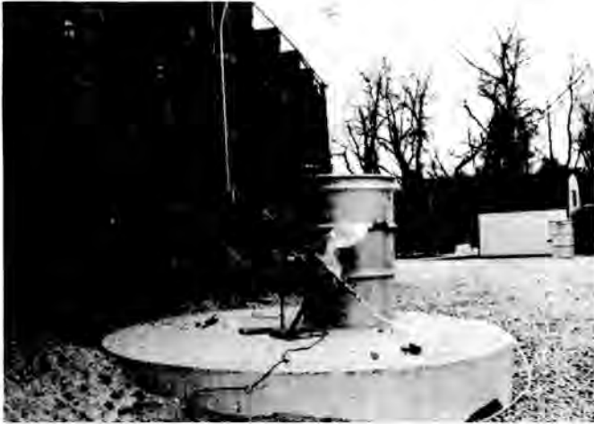
Fig. 4. Explosion test drum equipment setup.
