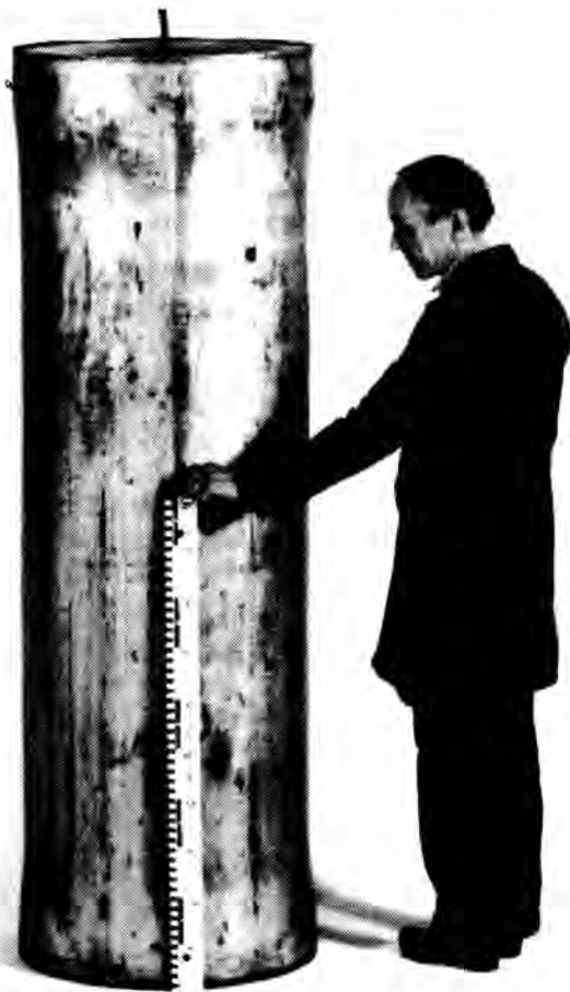
Fig. 1. The Swedish KBS-III container. In this design, fuel elements are encapsulated in copper powder which is hot isostatically pressed along with the 100-mm thick copper container body to produce a solid "monolith". (4)
