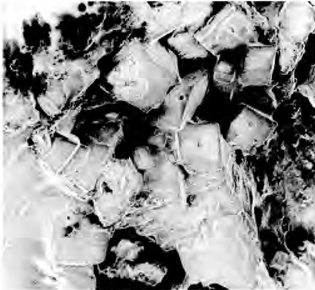
Fig. 7. A SEM Photomicrograph of a Solvent-Cleaned Surface of a Bitumen Waste Form Revealing Immobilized Nitrate Salts at a Magnification of 457X.
