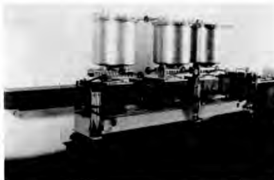
Fig. 2. A Photograph of the Bitumen Extruder/Evaporator.
