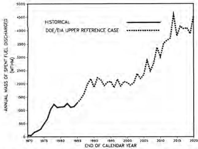
Fig. 5. Projected Mass (MTIHM) of Annual Commercial Spent Fuel Discharges for the DOE/EIA Upper Reference Case.
