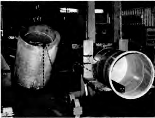
Fig. 2. Handling of Drums With Lost Concrete Shielding.
