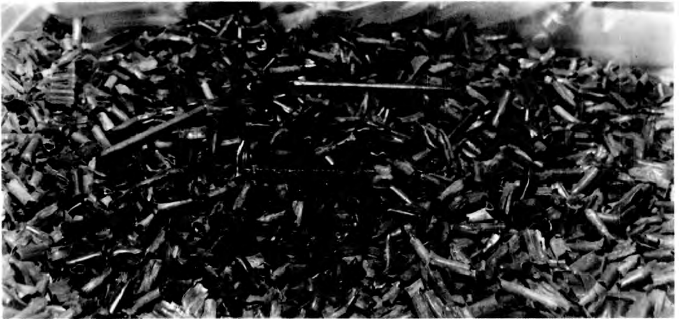
Fig. 1. General appearance of Obrigheim hulls recovered at La Hague reprocessing plant.
