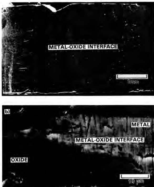
Fig. 5. Scanning Electron Micrographs of Cladding Samples With Thin Oxide From the 2-Month Experiment: a) Total specimen with well defined boundary between polished (right) and unpolished (left) areas, b) High magnification SEM micrograph of boundary showing oxide (dark) and metal (light) areas. Notice that the oxide-metal interface shows no topographical expression.
