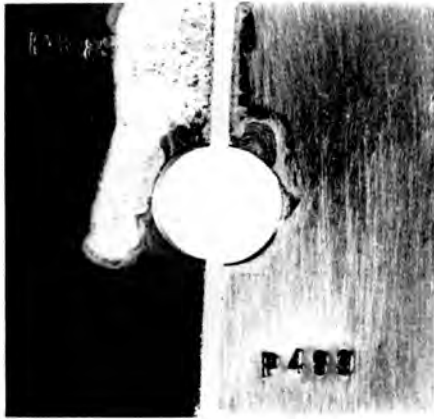
Fig. 4. Specimen Showing Crevice Corrosion Attack After Six Months Exposure. Half of specimen (on right) has been abraded to reveal attack near hole. Specimen was originally 36-mm square, with a 9.6-mm-diameter hole.
