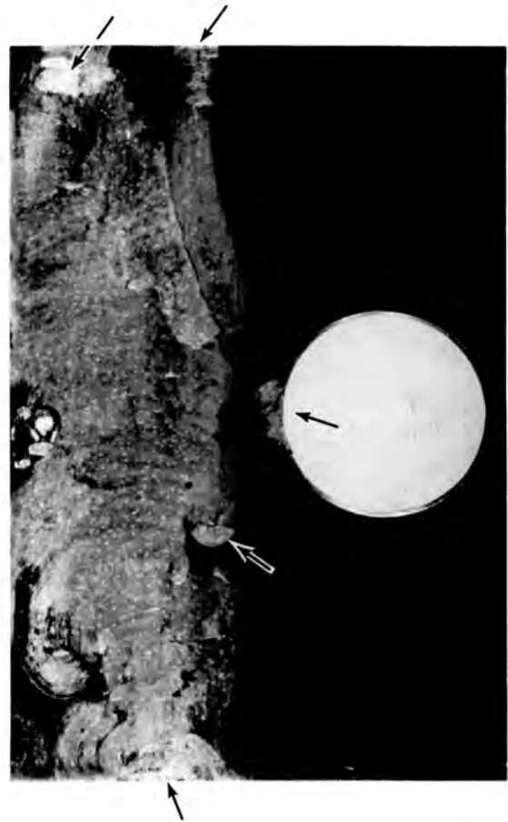
Fig. 6. Sites of Crevice-Corrosion Attack Under Corrosion Product ( TiO_2 ) Layer. Areas of severe attack are noted.
