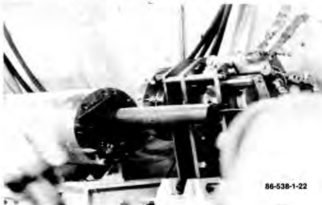
Fig. 2. TMI-2 core bore and casing being removed from shipping canister in TAN Hot Cell.
