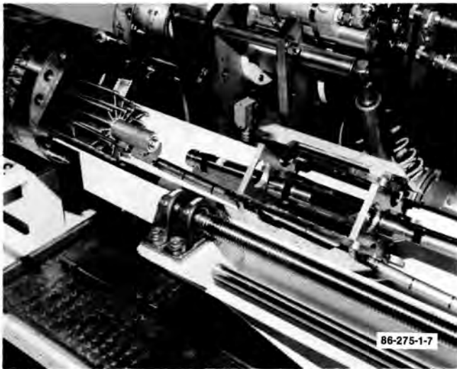
Fig. 17. View taken during trial operations showing hook tool aided by the video camera extracting a simulated control rod spider from a canister.
