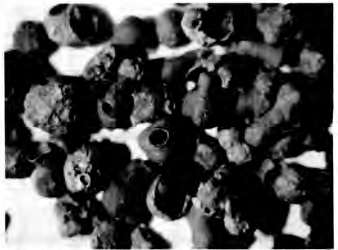
Fig. 1. Micrograph of a nickel ferrocyanide prepared by slow growth on sodium ferrocyanide crystals (magnification X 15).
