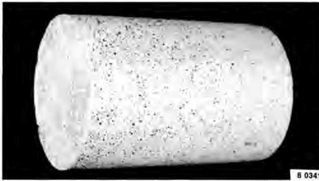
Fig. 5. Example of an EPICOR-II Resin Waste Form Solidified With Dow Polymer.
