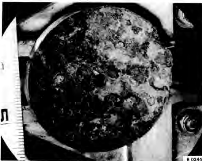
Fig. 7. Metallographic Section Removed From the wall of Liner PF-3, Showing Corroded Interior Surface.
