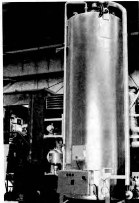
Fig. 9. Bitumen Storage Tank Showing Electric Controls
