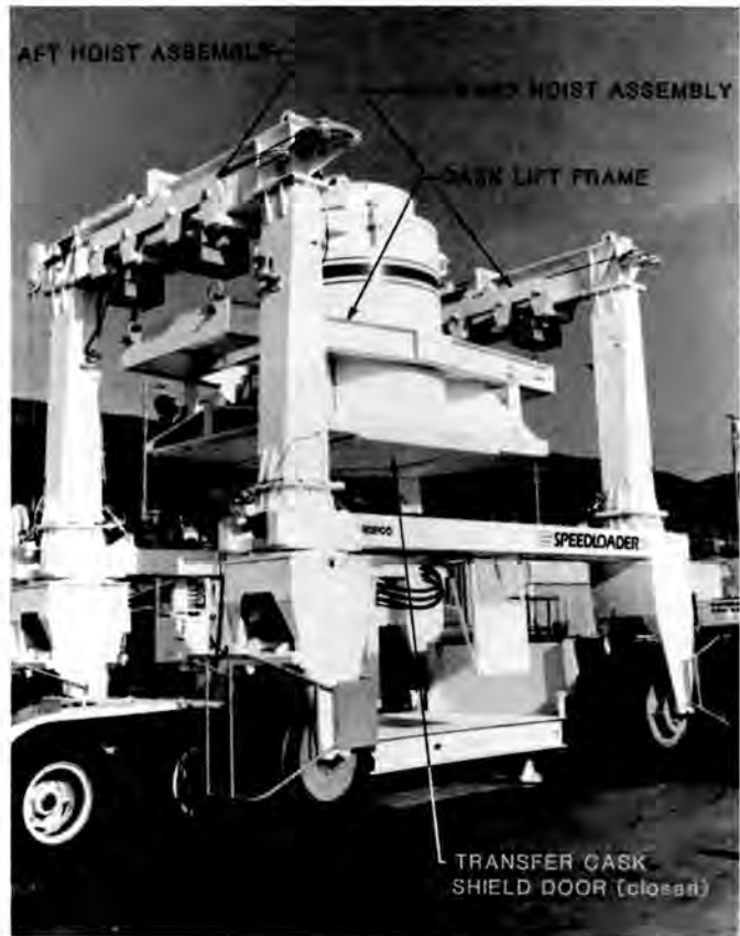
Fig. 4. Mobile Straddle Crane, Transfer Cask & Trailer Staged for Transfer Cask Loading
