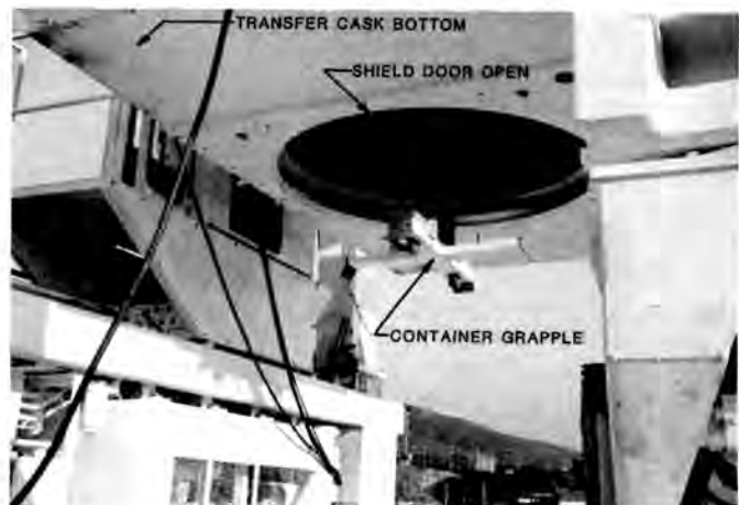
Fig. 5. Straddle Crane positioning transfer cask over container transfer area
