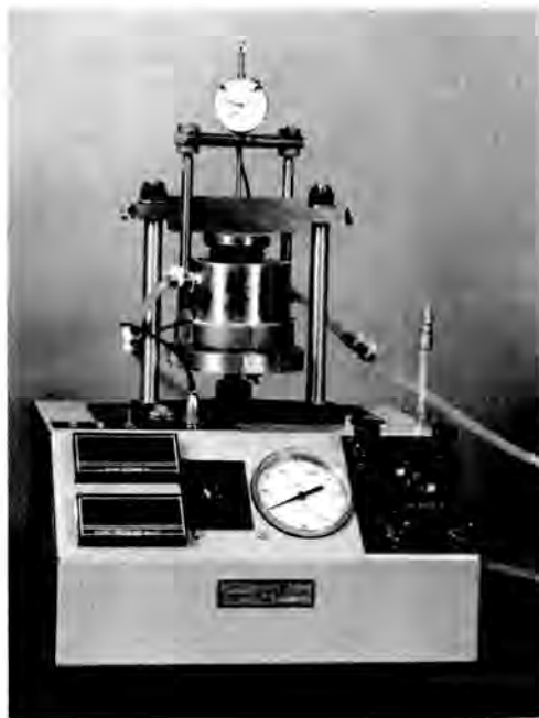
Fig. 1. Apparatus Used to Measure Consolidation of Simulated Single-Shell Tank Sludges
