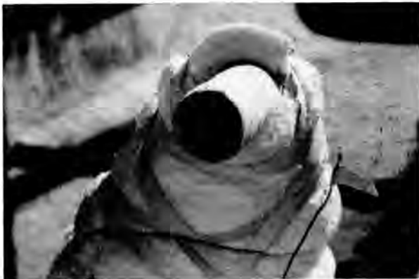
Fig. 5. Photograph of Transpiration Radiometers Following Insulation with Fiberfrax
