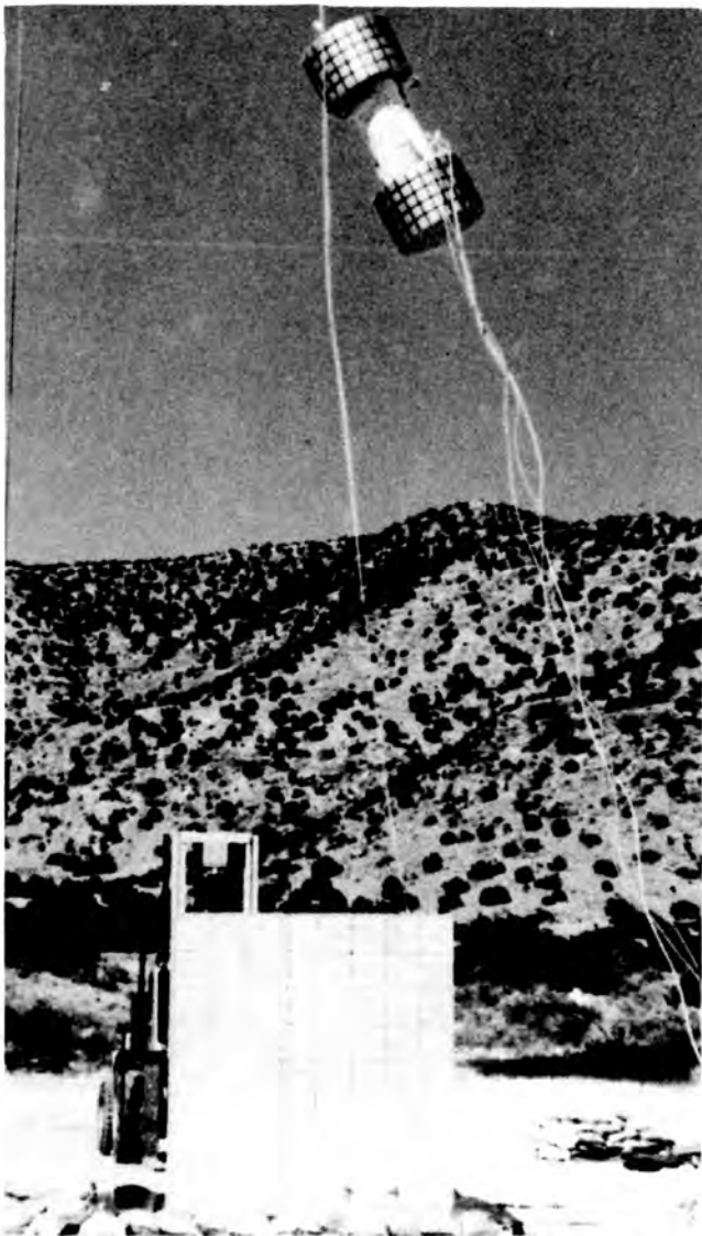
Fig. 11. Photograph of the 1/4-scale cask model being dropped from 30 ft during the oblique drop test at Sandia National Laboratories.
