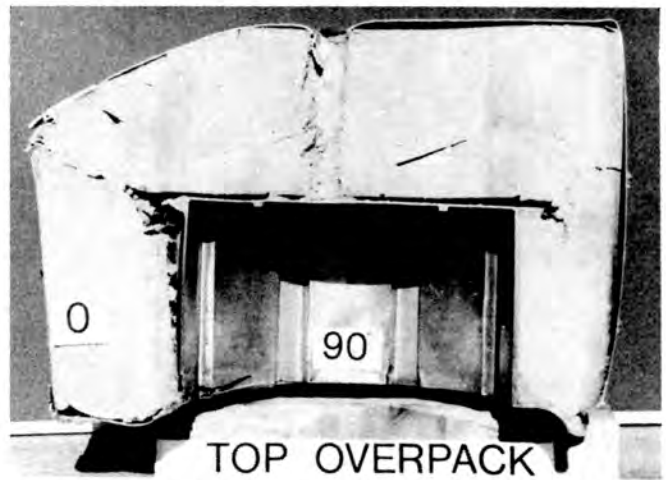
Fig. 13. Cutaway view of the damaged overpack of the 1/4-scale cask model after the tests pictured in Figs. 11 and 12.
