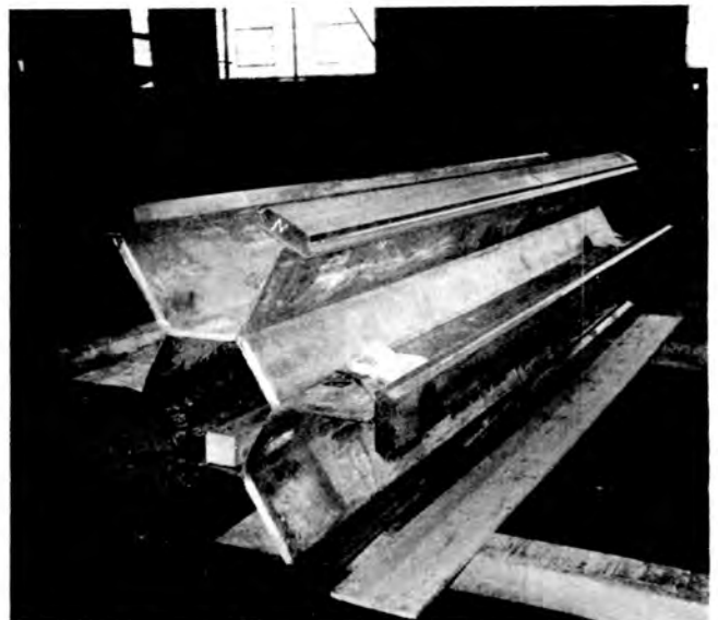
Fig. 18. Photograph of the hub and spoke arrangement of the inner vessel of the NuPac 125-B Rail Cask.
