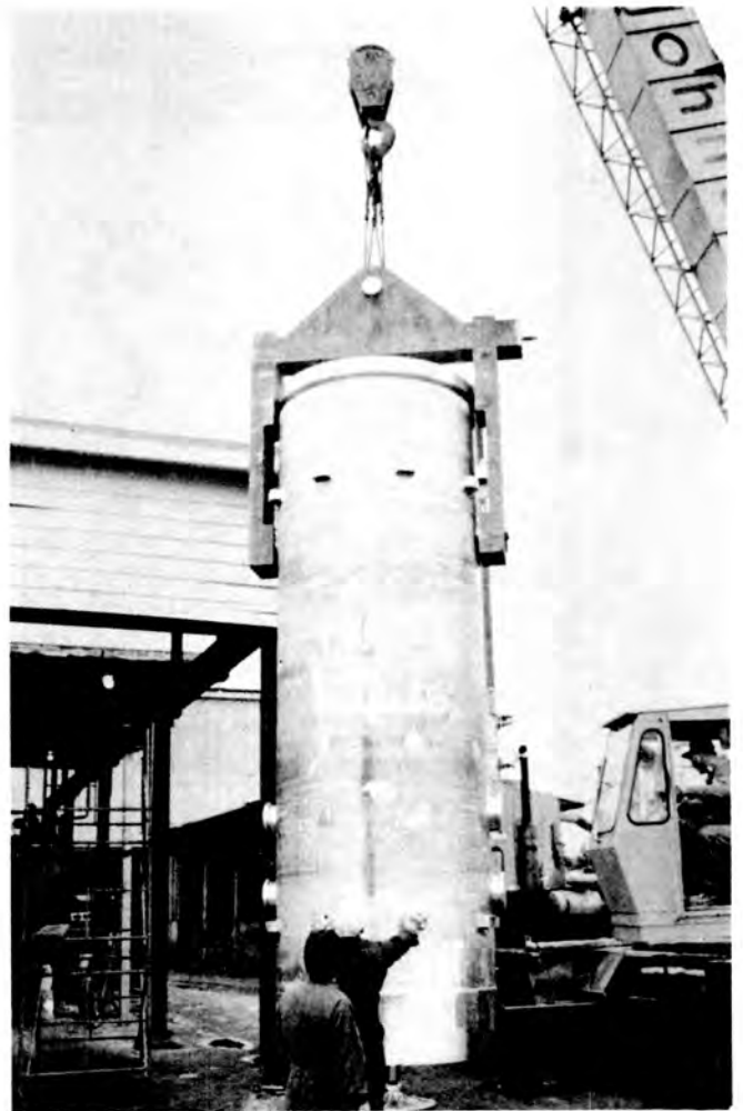
Fig. 17. Photograph of the outer vessel of the NuPac 125-B Rail Cask.
