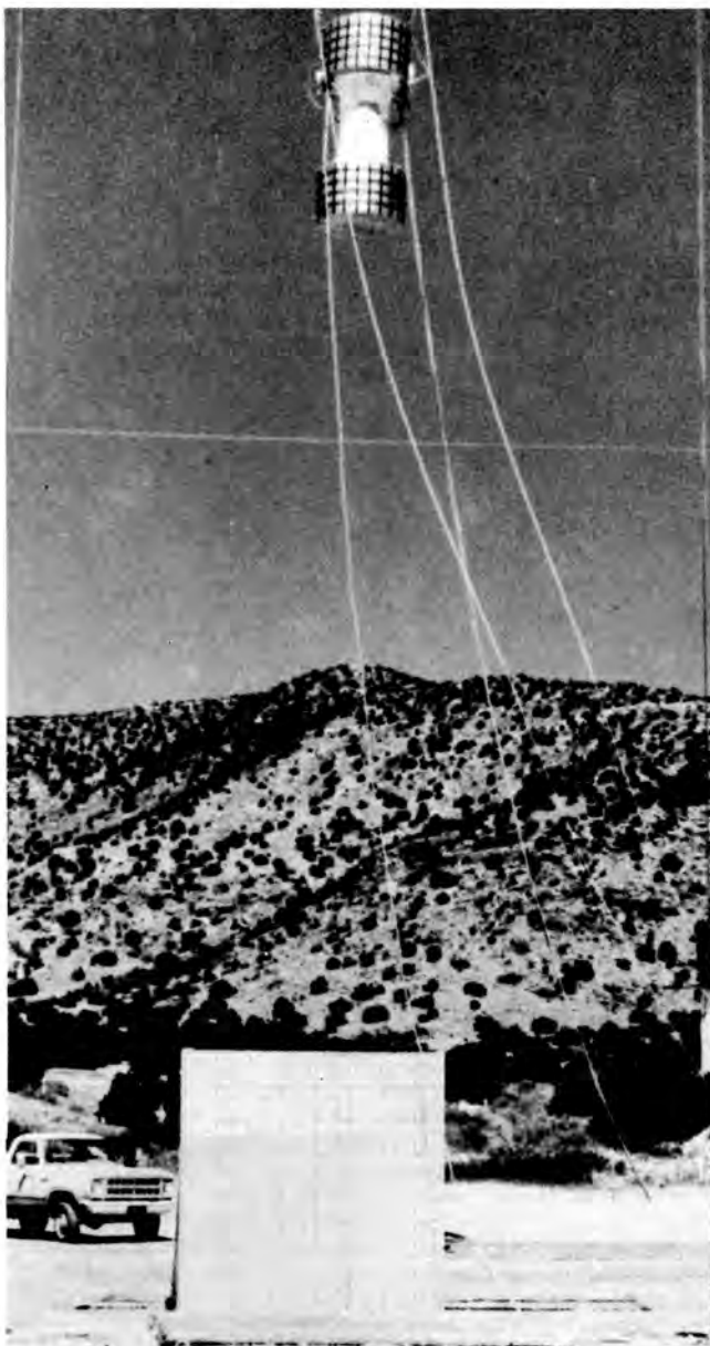
Fig. 9. Photograph of the 1/4-scale model of the NuPac 125-B Rail Cask during a 30-ft, end-on drop test at Sandia National Laboratories.
