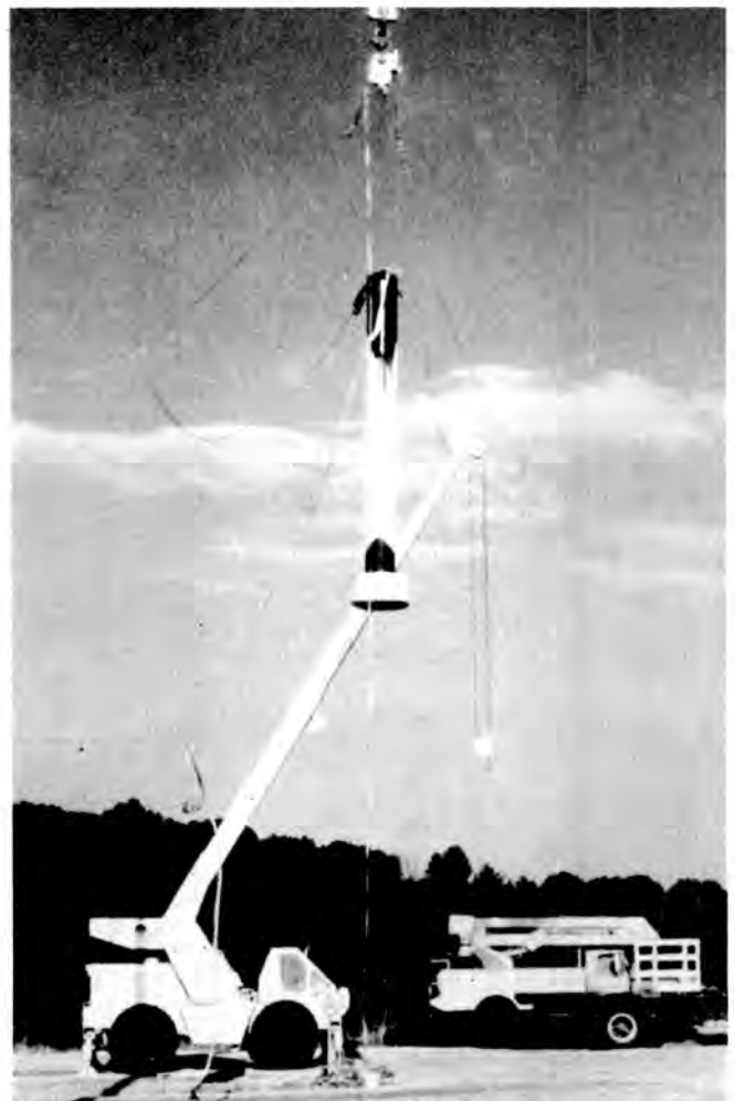
Fig. 10. Full-scale model of the TMI core debris canister before drop testing at Oak Ridge National Laboratory.
