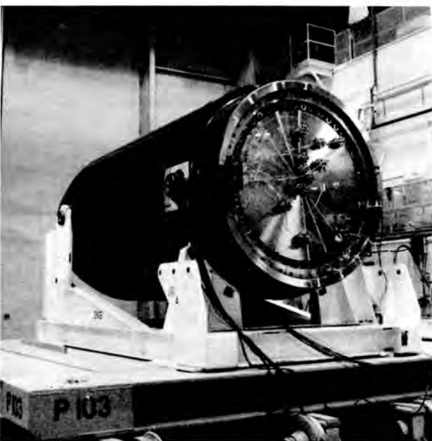
Fig. 2. Horizontal Testing of First Storage Cask (Castor V/21).
