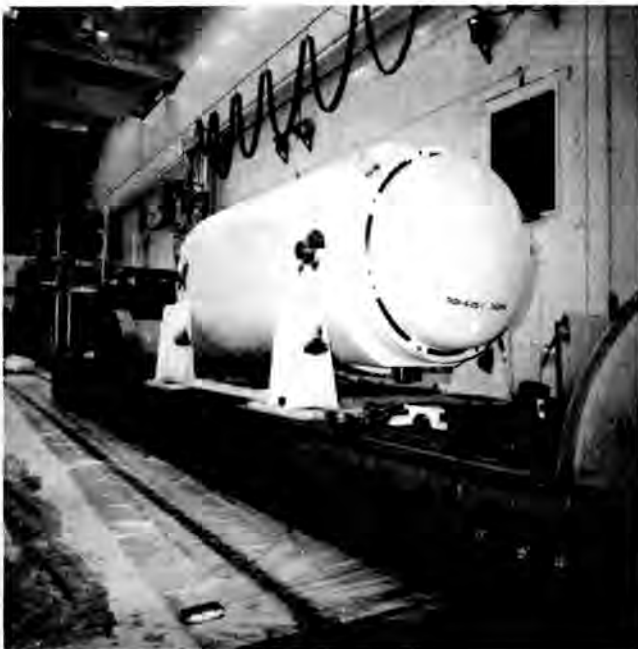
Fig. 3. Second Storage Cask (TN-24P).
